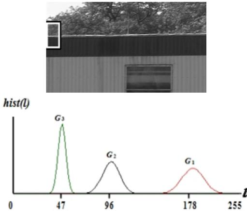
**Figure 4. (a) Rooftop that can be easily mistaken for a wire (thin bright line at the top of the roof). (b) Profile corresponding to the boxed area shown in (a). The large separation of the means indicates the profile at both sides of the edge is quite**
