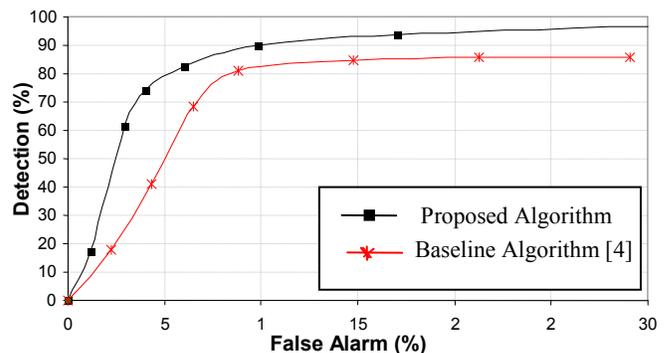
**Figure 5. Wire detection performance ROC, comparing previously published algorithms and proposed method.**
