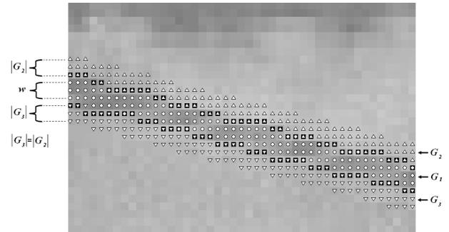
Figure 3. Profile estimation for the wire shown in Figure 2-b. The black squares represent edge pixels. The Gaussian model profile consists of 3 regions: the wire (shown in circles), and two other regions corresponding to the wire background (shown with straight and inverted triangles respectively).
